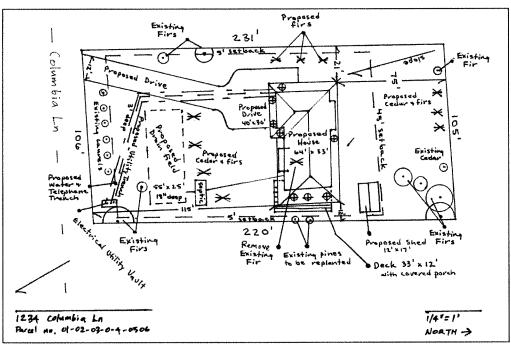
**EXAMPLE SITE PLAN:** The site plan must include all items listed in the site plan checklist (see pp. iv and v).
